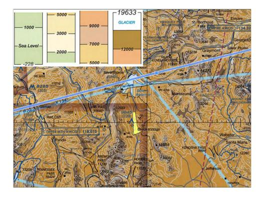
Here is a close-up of the same route. (Click) Terrain elevation is shown with specific colors on the sectional chart.
