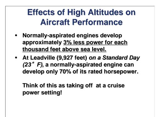
In order to attain the normal indicated airspeed required for rotation at Leadville, the airplane's true airspeed will be 20% greater than at sea level. A normally aspirated engine, is putting out 30% less horsepower than at sea level, and you have two factors working against you.
