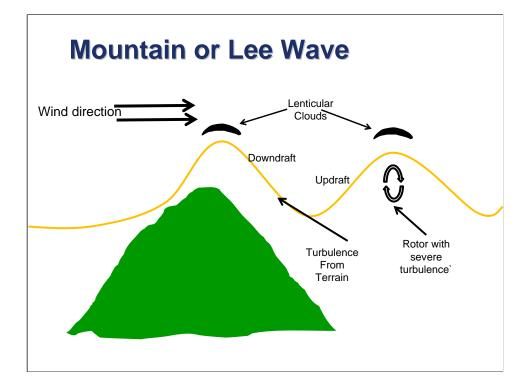
During a mountain wave event, there are strong up and down drafts downwind from the ridges. The downdrafts in even moderate mountain waves exceed 1000 feet per minute, making it difficult or impossible to cross the ridge. Rotors are caused by the wind shear and rotating moment underneath the crest of a mountain wave. The rotors will cause severe or greater turbulence and must be avoided.
