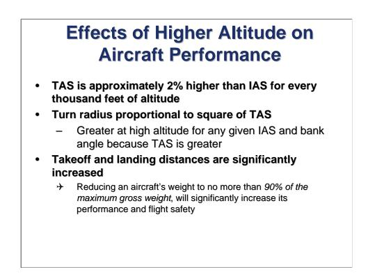
An <u>indicated</u> airspeed of 80 knots would be approximately 96 knots <u>true airspeed</u> at 10,000 feet above sea level.
