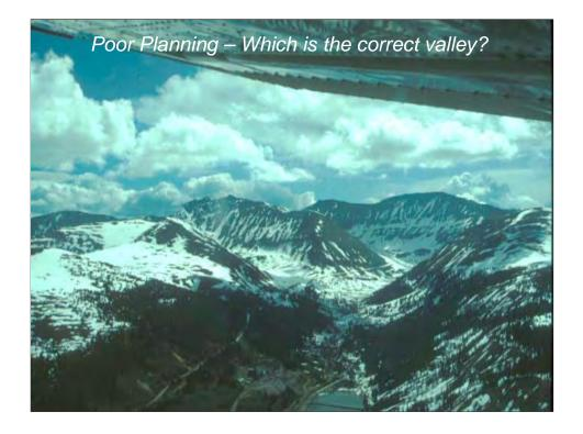
Doing adequate preflight planning will give you the correct heading to expect when picking the right valley to fly through. Making the wrong choice could get you into a position from which you can't escape. In this case, there are at least four valleys you might take, but only one is correct. The other three quickly become box canyons with rapidly rising terrain that you wouldn't be able to out-climb or turn around in.
