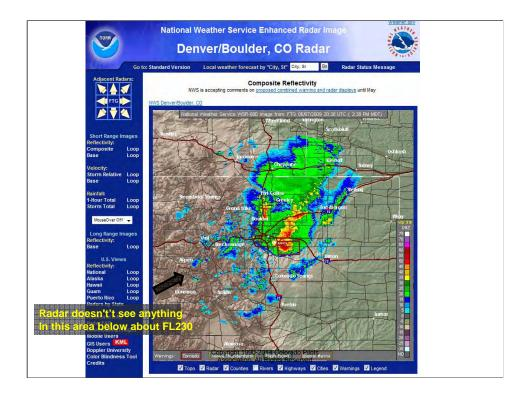
Many of us are now using radar on our tablet device while in flight. However, radar and mountains don't mix very well. For example, the Denver NEXRAD system can't see anything below about FL230 over the central part of the state. You may not be seeing the complete picture because of these limitations.
