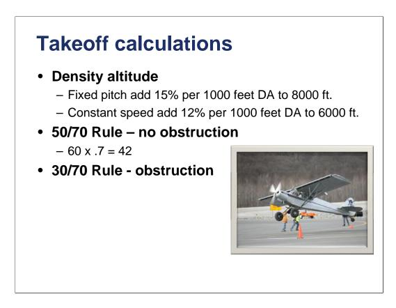
Here are some rules of thumb when making takeoff calculations.
