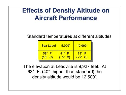
Assuming a standard altimeter setting, anything above standard temperature at your elevation means your density altitude is above the field elevation.
