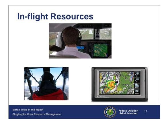
You may be piloting a plane with the latest glass cockpit equipment that displays traffic and weather. But you might be flying older technology aircraft with a mobile device for navigation and weather data assistance. Either way it's nice to confirm what you're seeing with weather specialists or controllers on the ground.
