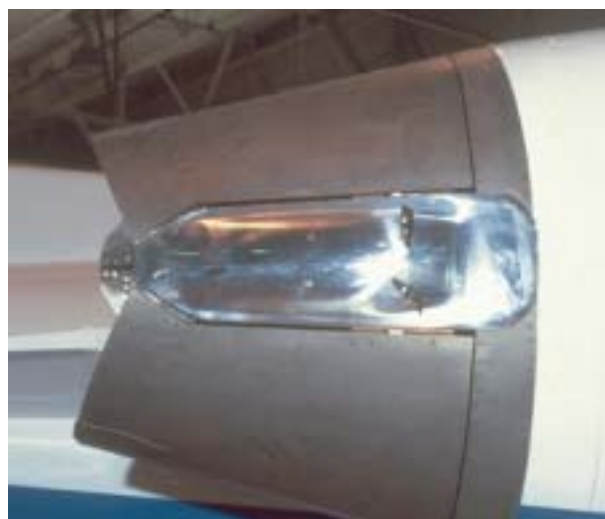
Figure 7-22. Thrust Reverser (Dee Howard TR 4000)
