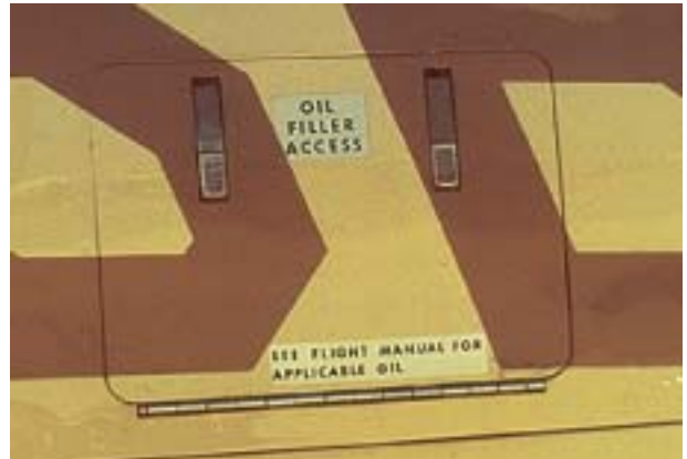
41. RIGHT ENGINE OIL QUANTITY —CHECK FILLER CAP AND ACCESS DOOR—SECURE
