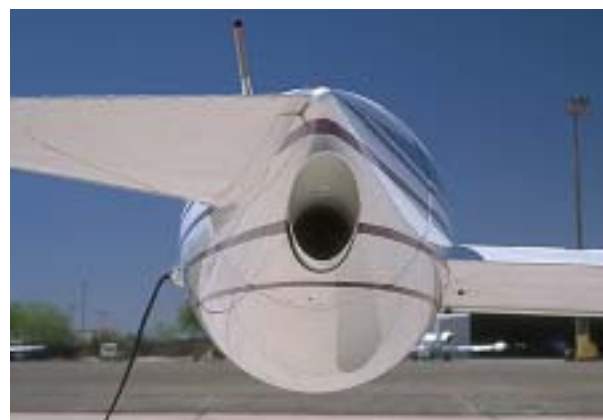
72. LEFT TIP TANK FUEL JETTISON TUBE—CLEAR OF OBSTRUCTIONS
