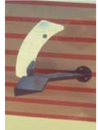
12. RIGHT STALL WARNING VANE —FREEDOM OF MOVEMENT, LEAVE IN DOWN POSITION
