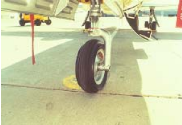
8. NOSEWHEEL AND TIRE —CONDITION AND NOSE GEAR UNLOCK FORWARD
