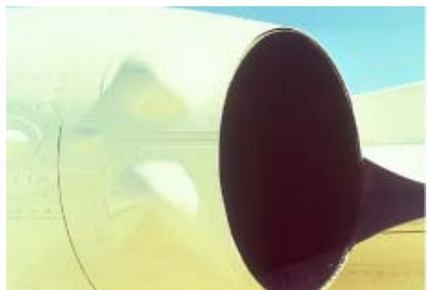
66. LEFT ENGINE TRUST REVERSER —CONDITION AND STOWED (AERONCA)
