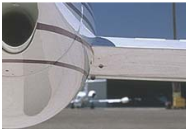
71. SCUPPER (UNDERSIDE OF LEFT WING AFT)— CLEAR OF OBSTRUCTIONS, NO FUEL LEAK
