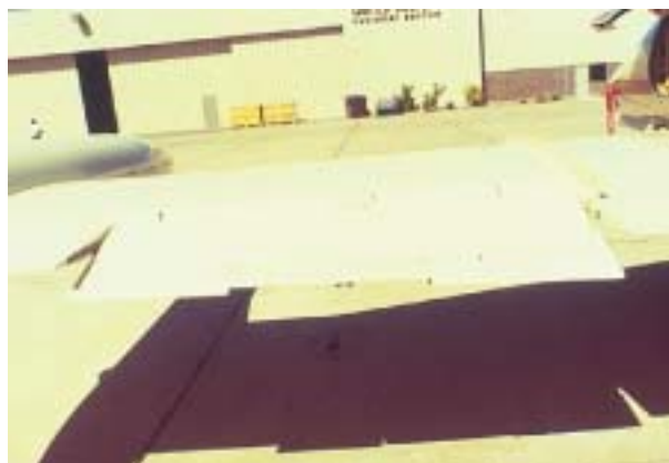
70. LEFTAILERON—CHECK FREE MOTION, BALANCE, AND TRIM LINKAGE, AND BRUSH SEAL CONDITION
