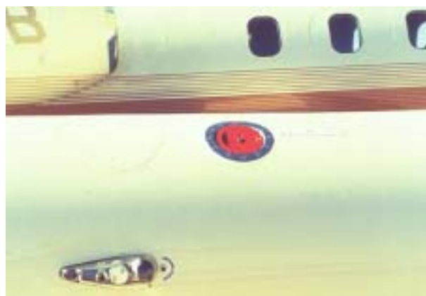
34. RIGHT TIP TANK FUEL CAP—CONDITION AND SECURE
