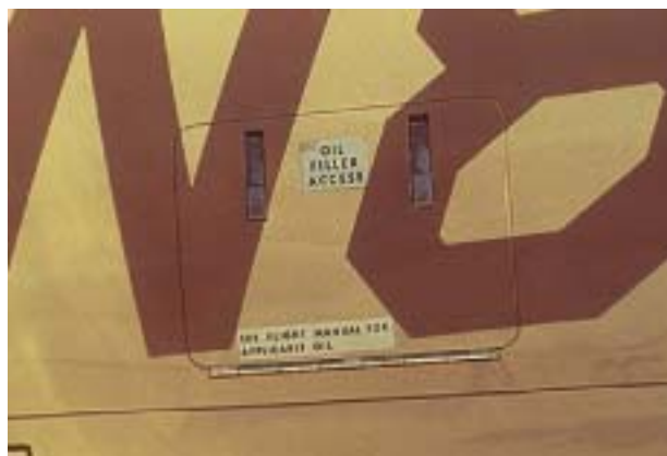
68. LEFT ENGINE OIL QUANTITY—CHECK FILLER CAP AND ACCESS DOOR—SECURE
