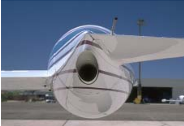
37. RIGHT TIP TANK FUEL JETTISON TUBE —CLEAR OF OBSTRUCTIONS
