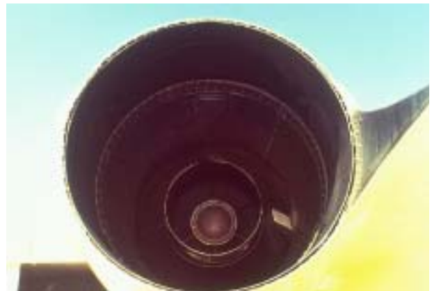
65. LEFT ENGINE TURBINE EXHAUST AREA— CONDITION, CLEAR OF OBSTRUCTIONS AND BLOCKER DOORS STOWED (AERONCA)
