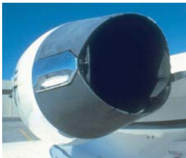
Figure 7-22. Thrust Reverser (Dee Howard TR 4000)
