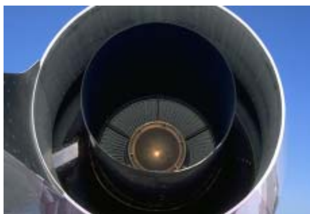
44. RIGHT ENGINE TURBINE EXHAUST AREA—CONDITION, CLEAR OF OBSTRUCTION, BLOCKER DOORS STOWED (AERONCA)
