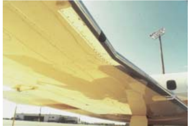
27. RIGHT WING ACCESS PANELS (UNDERSIDE OF WING)—CHECK FOR FUEL LEAKAGE
