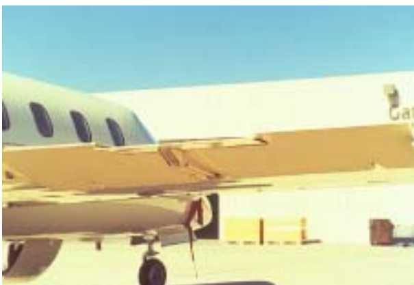
39. RIGHT AILERON —CHECK FREE MOTION, BALANCE TAB LINKAGE, BRUSH SEAL CONDITION
