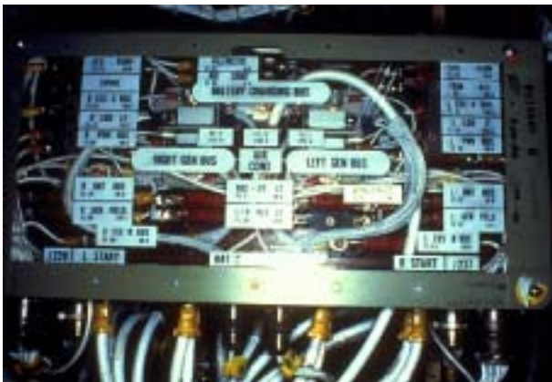
49. TAILCONE INTERIOR—CHECK FOR FLUID LEAKS, SECURITY, AND CONDITION OF INSTALLED EQUIPMENT
