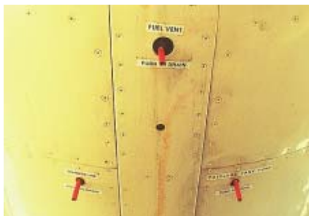
46. FUEL VENT DRAIN VALVE, TRANSFER LINE DRAIN VALVE, FUSELAGE TANK SUMP DRAIN VALVE—DRAIN
