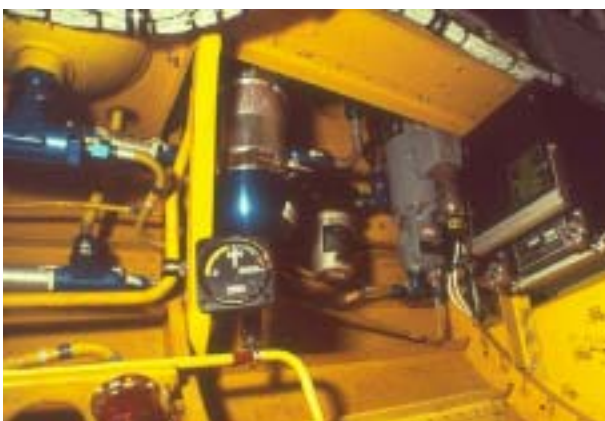
49A. TAILCONE INTERIOR—CHECK FOR FLUID LEAKS, SECURITY, AND CONDITION OF INSTALLED EQUIPMENT HYDRAULIC ACCUMULATOR AIR CHARGE—750 PSI MINIMUM
