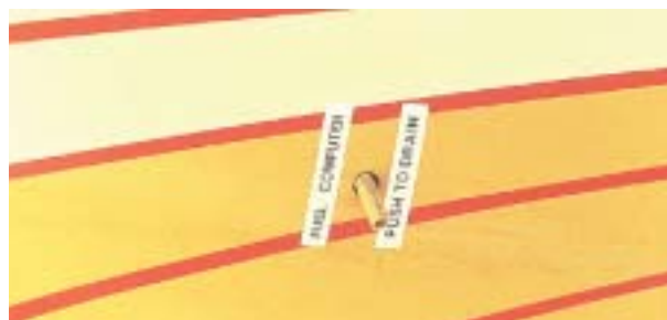
55. RIGHT FUEL COMPUTER DRAIN VALVE—DRAIN (DRAIN VALVES ARE RECESSED ON AIRPLANES EQUIPPED WITH DRAG CHUTE.)
