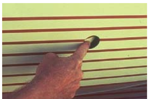
42. RIGHT ENGINE OIL BYPASS VALVE INDICATOR —CHECK, NOT EXTENDED
