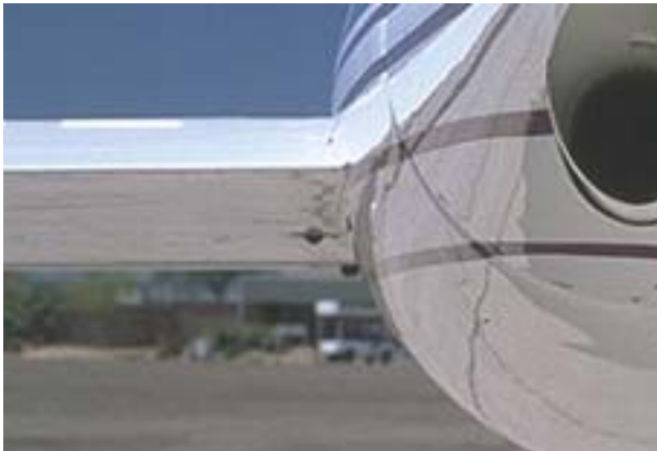
38. SCUPPER (UNDERSIDE OF RIGHT WING AFT) —CLEAR OF OBSTRUCTIONS, NO FUEL LEAKAGE
