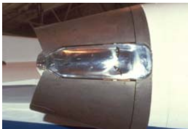
43A. RIGHT ENGINE THRUST REVERSER—CONDITION AND STOWED (DEE HOWARD)
