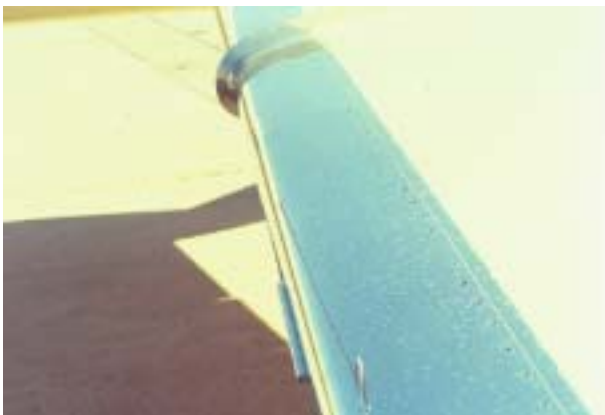
26. STALL STRIP, WING LEADING EDGE, AND STALL FENCE—CONDITION
