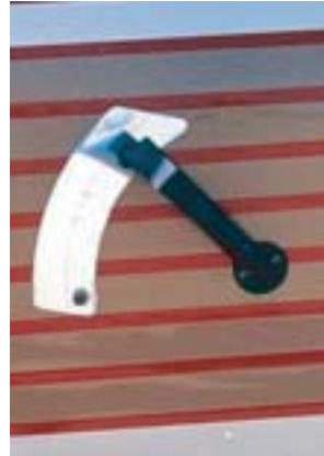
12. RIGHT STALL WARNING VANE —FREEDOM OF MOVEMENT, LEAVE IN DOWN POSITION
