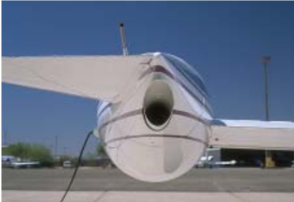
73. LEFT TIP TANK FIN AND STATIC DISCHARGE WICKS (2)—CONDITION
