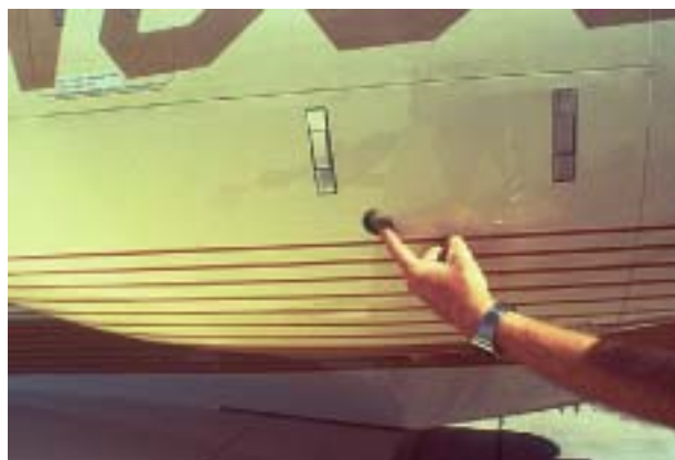
67. LEFT ENGINE FUEL BYPASS VALVE INDICATOR— CHECK, NOT EXTENDED
