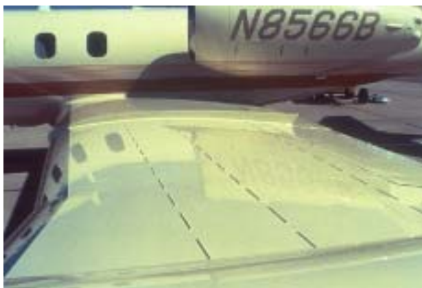
80. VORTEX GENERATORS OR BOUNDARY LAYER ENERGIZERS—CONDITION
