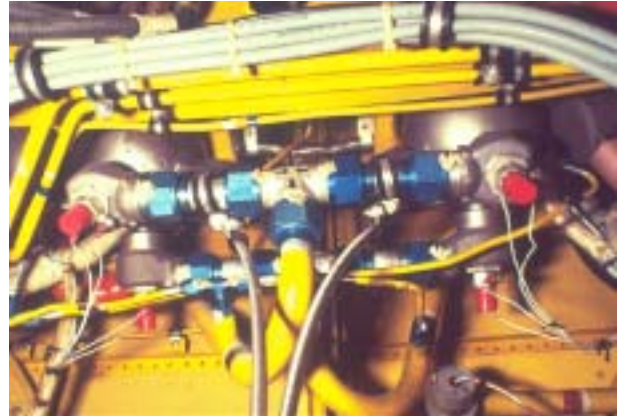
49B. TAILCONE INTERIOR—CHECK FOR FLUID LEAKS, SECURITY, AND CONDITION OF INSTALLED EQUIPMENT
