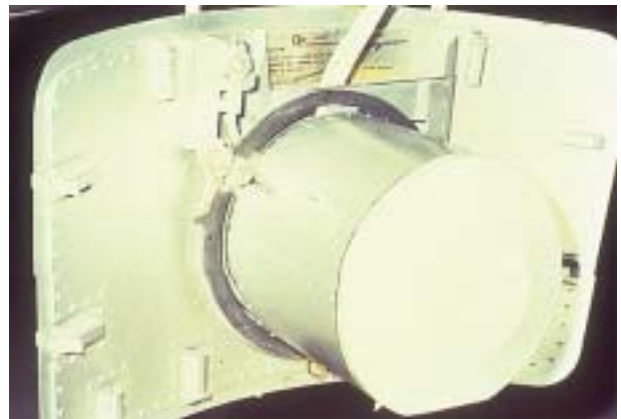
50. DRAG CHUTE—CHECK FOR PROPER INSTALLATION
