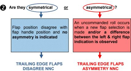
The flaps asymmetry can be caused by a mechanical failure in the flaps drive mechanism or a
