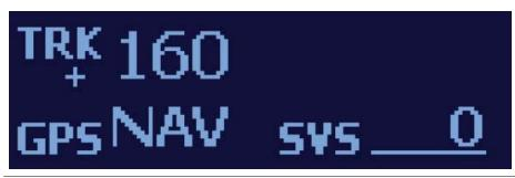
**Vertical Speed** can be adjusted by a momentary press and release of the KNOB to move the cursor under the number next to SVS, and then rotating the KNOB.
